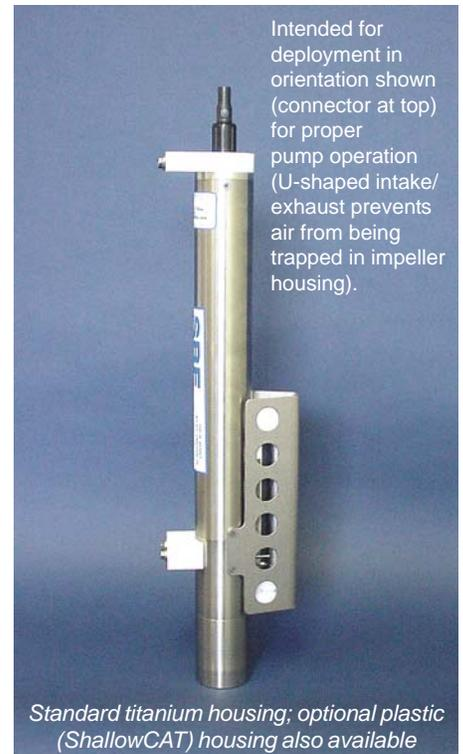
Intended for deployment in orientation shown (connector at top) for proper pump operation (U-shaped intake/exhaust prevents air from being trapped in impeller housing).
